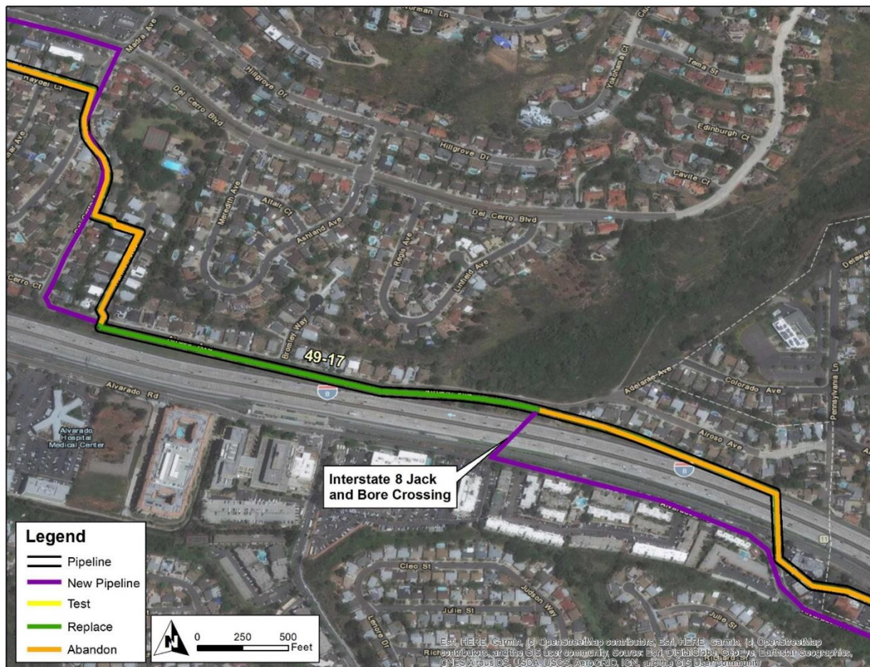
Figure 6: Satellite Image of Interstate 8 Jack and Bore Crossing
