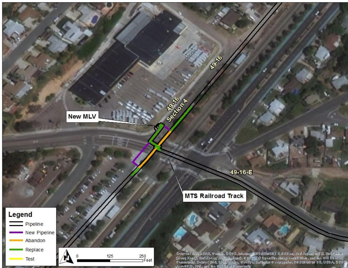
Figure 9: Satellite Image of Supply Line 49-16 Section 4 Replacement Project
