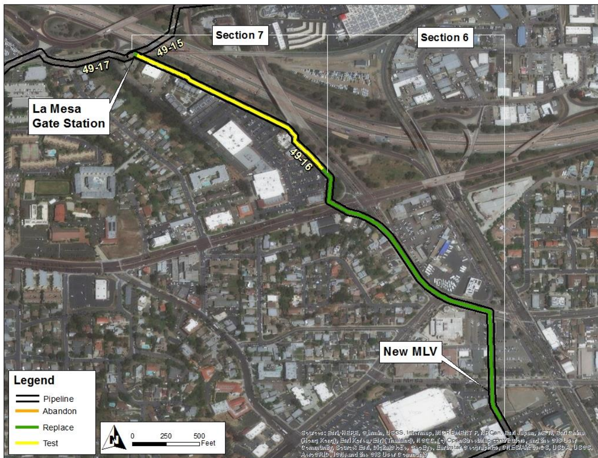
Figure 13: Satellite Image of Supply Line 49-16 Replacement and Hydrotest Project, Section 6 and Section 7
